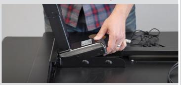
STEP 8 Connect the hand controller cable to Leg1 as shown.
