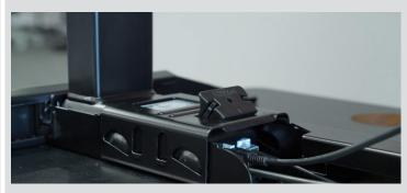
Repeat the same process on the other side for Leg 2, then plug in the other end of the 6 port cable into Leg 2 as shown.
