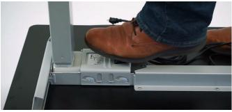
STEP 18 Screw down the control box in the center of the desk and between the crossbar and back edge of the desktop.
