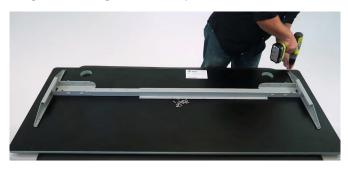
Next, finish securing the desktop to the base by inserting all remaining screws.
