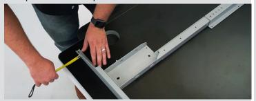
**NOTE:** The Lander Base is a C-Leg mechanism and is designed to be mounted closer to the back edge of the desktop. Ensure your base is aligned properly on the desktop as shown in the diagram.
