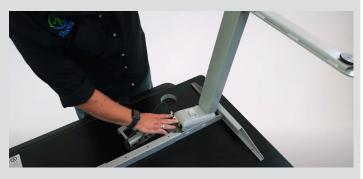
STEP 16 Step down firmly on the clamp lock to fix the lock in place. This may require some force, wear a stiff shoe/boot and apply standing weight forcing down.
