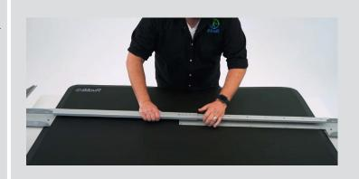
Extend the assembly until the STEP 5 short end of the top support arm on the crossbar assembly is 1.5" from the back edge of the desktop.
