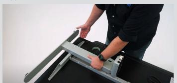
STEP 11 Place the motor end of the leg into the motor housing.
