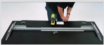
Now that you are ready to screw the assembly to the desktop. First secure opposing corners of the assembly to ensure that the assembly remains aligned during the install process.
