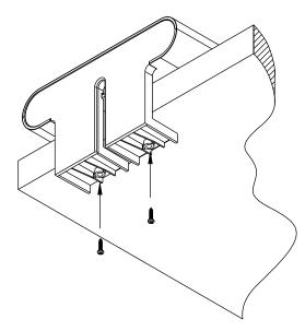
To prevent damage to table top please note: Assuming a desktop at least 3/4" thick, drill pilot holes a maximum of 1/2" deep to keep from drilling through the table top. Over tightening of screws during installation or adjustments can damage the product and affect the function and warranty.
