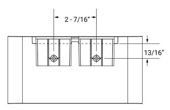
Use screws (not provided) to mount the Ellipse into position as shown.
